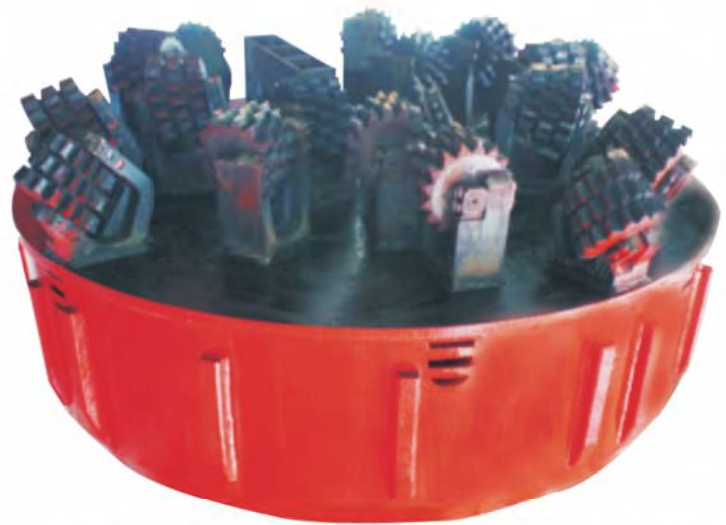
φ3.5m full section shaft welding hob drill bit
