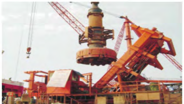
φ3.4m welding hob bit be used on bridge site construction
