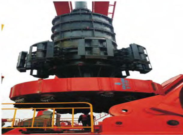
φ4.5m pile bit of the Pingtan sea bridge, China
