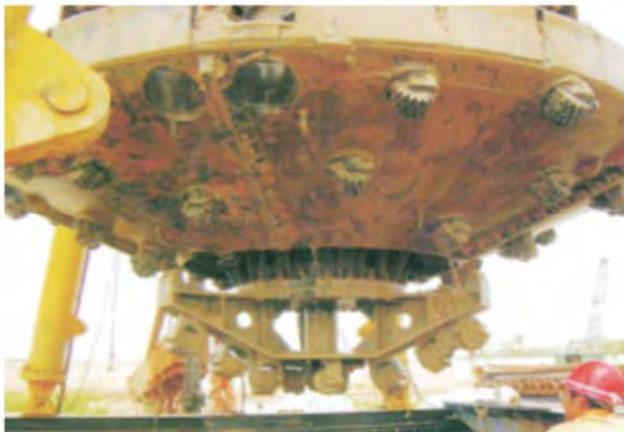
3° welding gear hob drill bit be used on the building site
