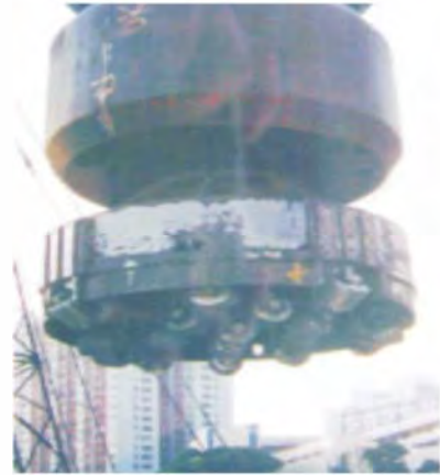
Ball gear hob drill bit on the building site of Hong Kong
