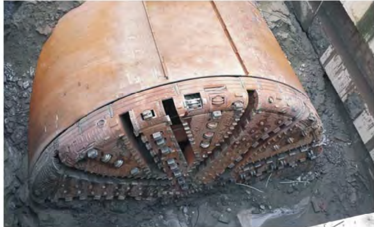
Shield machine tool in Nanjing latitude three passing River Tunnel
