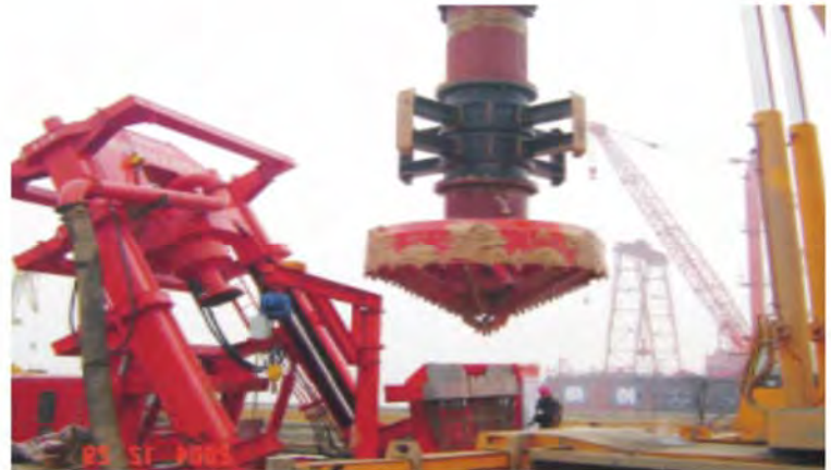
φ3.4m scraper drill bit be used on bridge site construction
